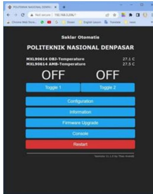
**Gambar 6. Interface Web Saklar Otomatis**
