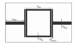
Fig. 3. SLR Filter Design
