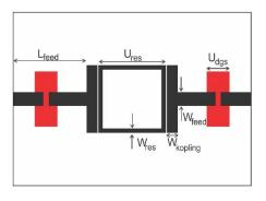
Fig. 4. SLR Filter with DGS
