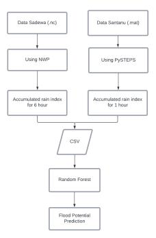
Figure 7. Machine learning workflow block diagram
