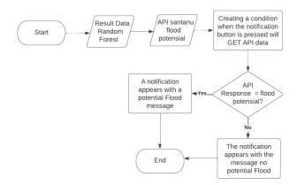
Figure 3. Flowchart Notification Flood Prediction
