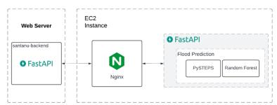
Figure 5. Block diagram of the machine learning server
