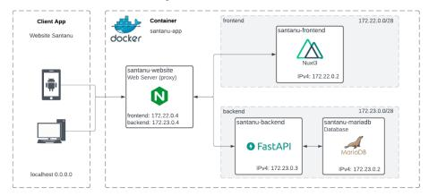
Figure 4. Block diagram of the web server
