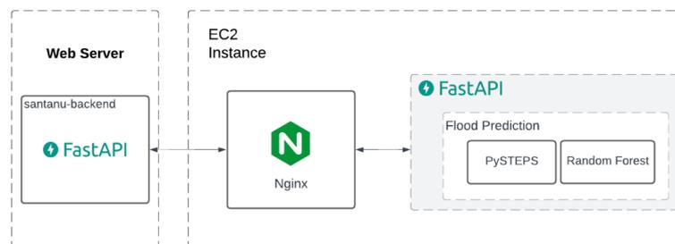
Figure 5. Block diagram of the machine learning server
