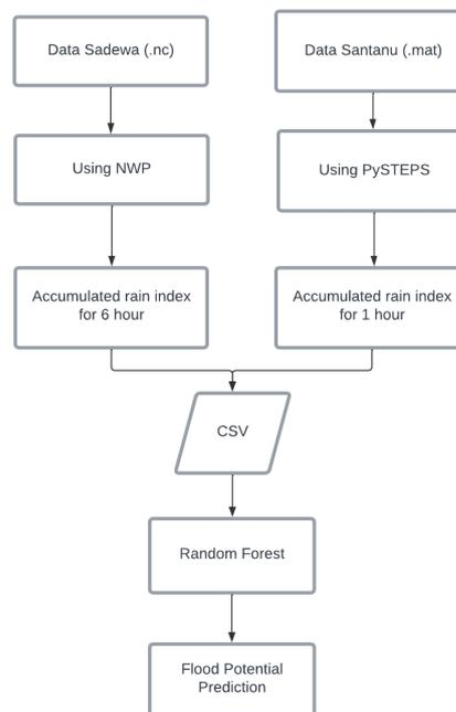
Figure 7. Machine learning workflow block diagram
