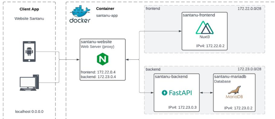
Figure 4. Block diagram of the web server
