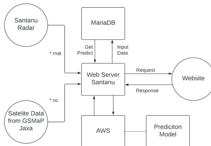
Figure 1. System Architecture Design
