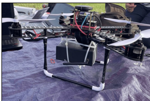
Figure 5. LoRa Gateway Installation on Autonomous Drones
