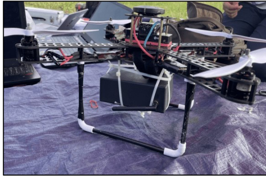
Figure 5. LoRa Gateway Installation on Autonomous Drones
