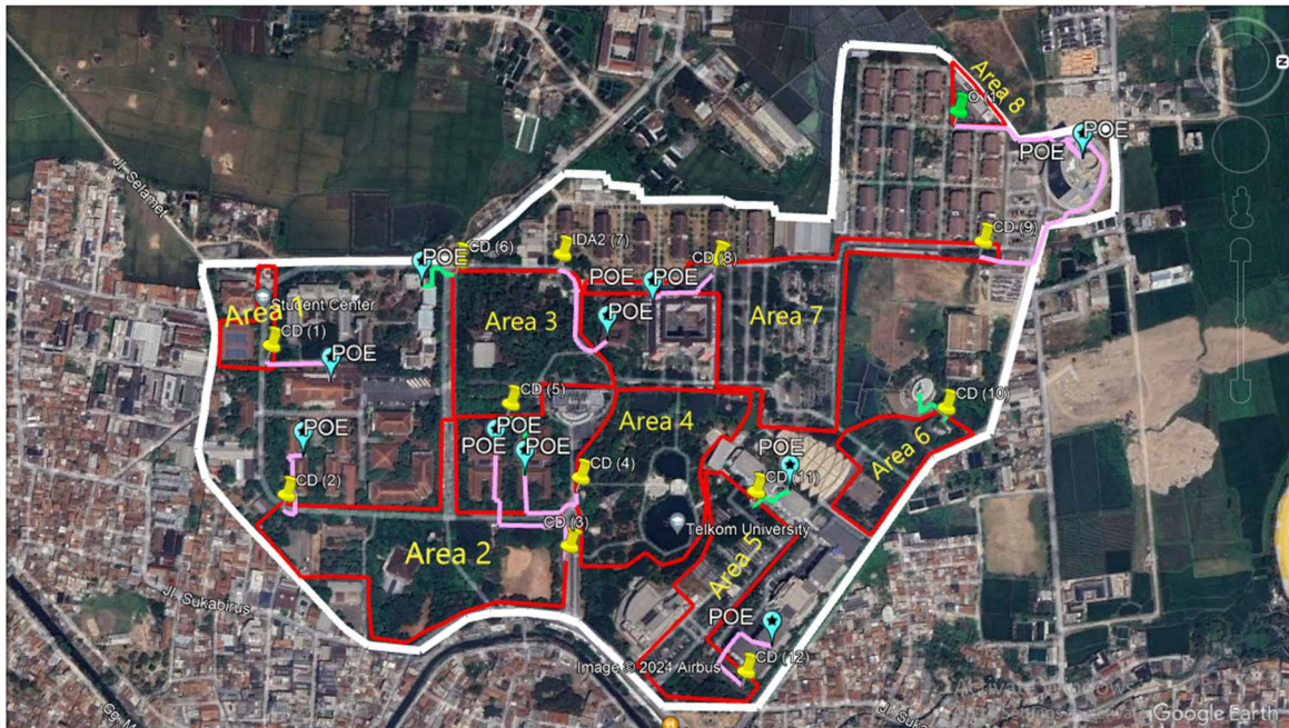
Figure 10. Scenario 4-C Transmission Cable Distribution Map
