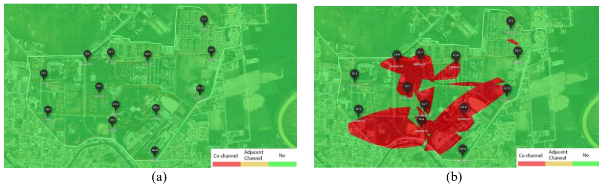
Figure 7. Heatmap of Simulated Interference in Frequency Band (a) 2.4 GHz and (b) 5 GHz
