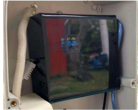
Gambar 6. Alat monitoring (SU: Suhu Udara, SA: Suhu Air, H: Kelembapan)
