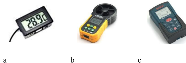
Gambar 2. (a) Thermometer & Hygrometer Digital, (b) Anemometer Digital, (c) Meteran Digital Sumber : Dokumentasi Peneliti, 2022
