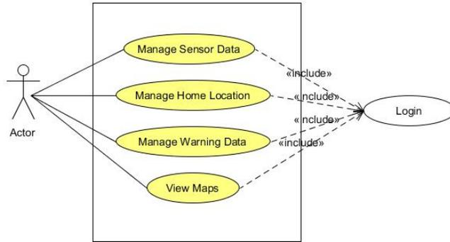
Figure 6 Use Case Diagram
