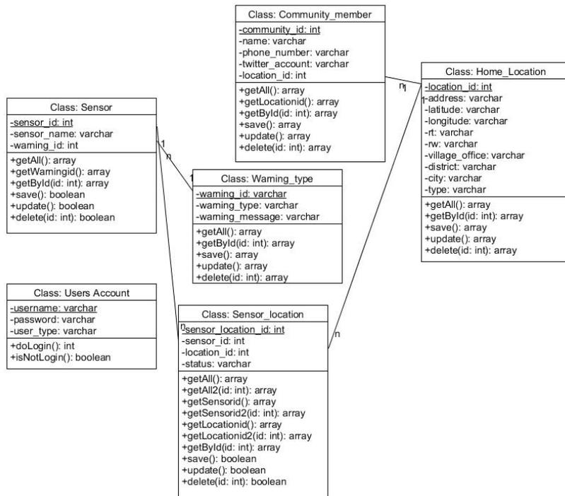
Figure 7 Class Diagram
