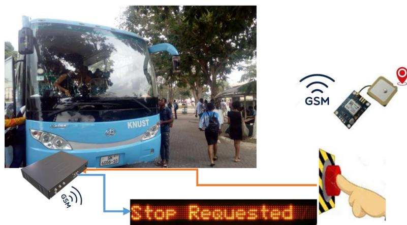
Figure 1 PDSCV System Architecture
