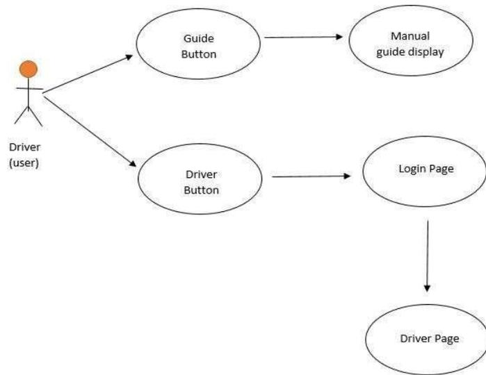
**Figure 5** PDSCV System Software Use Case Diagram
