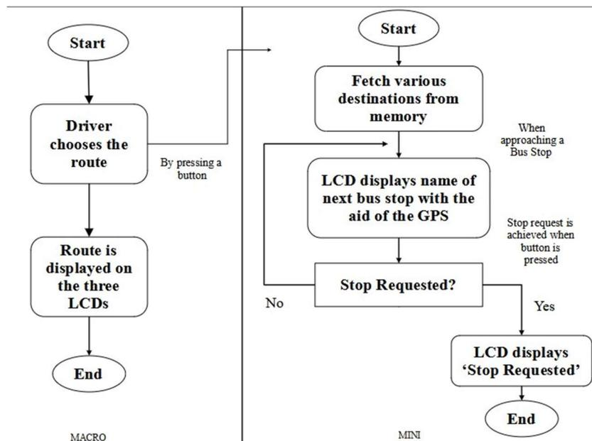
Figure 4 PDSCV System Workflow
