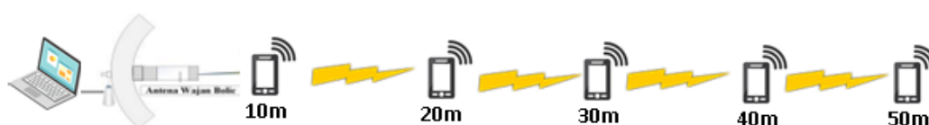
Figure 6. Wokbolic antenna testing every 10 meters to 50 meters from the access point
