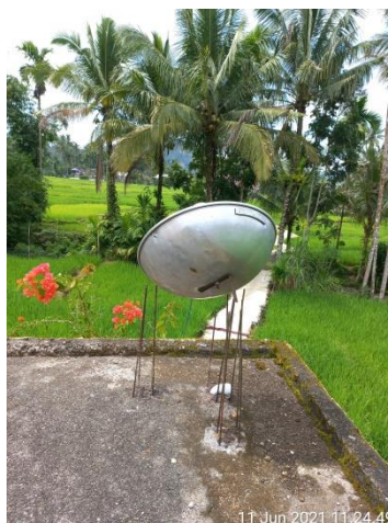
Figure 9. Wokbolic antenna implementation on smart agriculture
