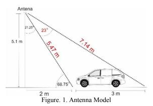
Based on above-mentioned system model, the antenna being designed should have a required half power beam width (HPBW) angle of 23° to cover the width of one gate lane.
