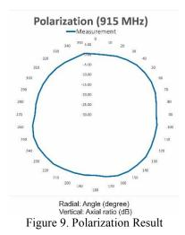
Looking at the results, the average axial ratio of the printed antenna appears at 1.39 dB. Besides, antenna with an axial ratio <3 dB perform a circular polarization [8], hence fulfilling required circular polarization parameter. The CP antenna would ensure a seamless reading process when RFID tags rotate in various phi ( $\phi$ ) angles. In fact, no power attenuation occurs when power from a tag is received.
