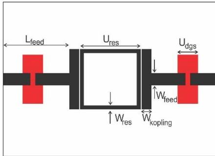
Fig. 4. SLR Filter with DGS
