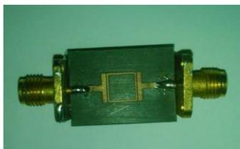
Fig. 6. Final Printed Filter (Top View)
