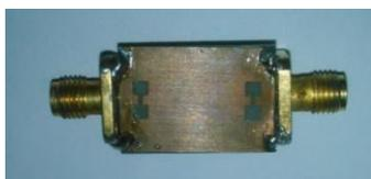
Fig. 7. Final Printed Filter (Rear View)
