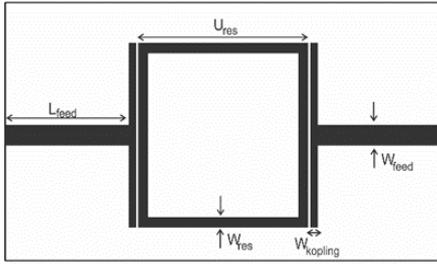
Fig. 3. SLR Filter Design
