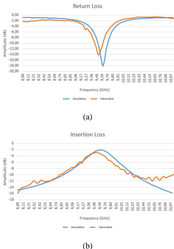
Fig. 8. (a) Return Loss Measurement result with DGS, and (b) Insertion Loss Measurement result with DGS
