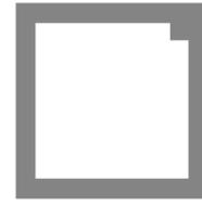
Fig. 2 Square Loop Resonator Shape
