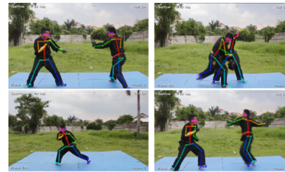
Fig. 3. OpenPose for skeleton readings in single subjects and two subjects, for example, pencak silat motions.
