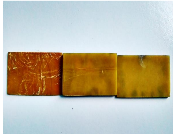
Fig. 7 an FR-4 Dielectric Material with thickness 1,6 mm (left), 3,2 mm (center), and 4,8 mm (right)
