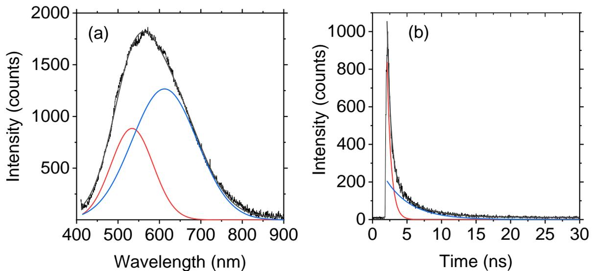
Fig. 4 (a) The photoluminescence and (b) the time resolved photoluminescence spectra of sub-micrometer WS<sub>2</sub>. The red and blue lines at (a) to show the Gaussian fits while the ones at (b) to show the exponential fits.
