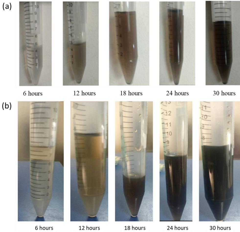
Fig. 1. The WS<sub>2</sub> solution as a function of fabrication time. The external voltage were (a) 3 V and (b) 4 V.
