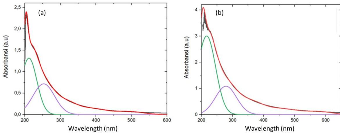
Fig. 3. The UV-VIS spectra of WS<sub>2</sub> solution after (a) 18 and (b) 30 hours electrochemical process. The laser excitation wavelength is 205 nm. Color lines are fitted with Gaussian function to show that the whole spectra consist of multiple peaks centered in various wavelengths.
