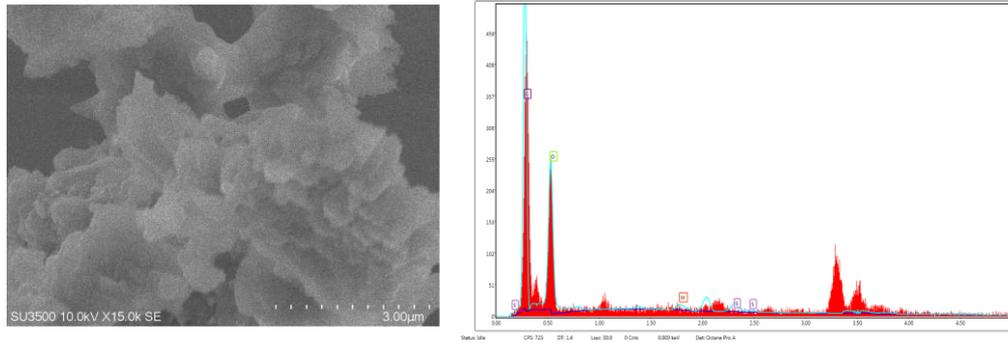
Fig. 3. The typical morphology of WS<sub>2</sub> deposited on ITO/PET
