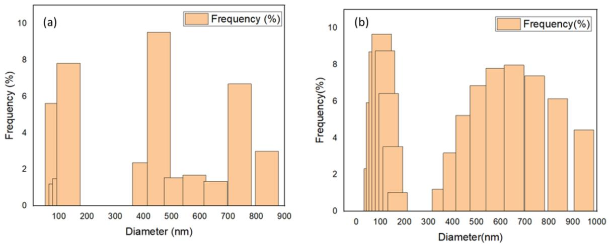
Fig. 2. The particle size distribution of WS<sub>2</sub> solution after (A). 18 and (B) 30 hours electrochemical process.
