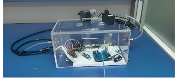
Fig. 3. Vehicle emission testing chamber.
