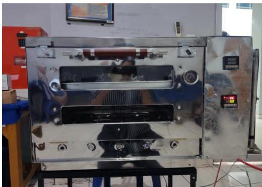
Fig. 2. A dehydrator with integrated PID control
