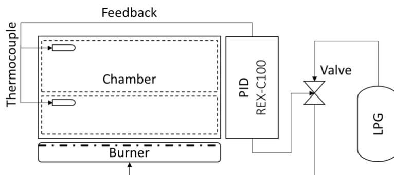
Fig. 1. Instrumentation system design of dehydrator
