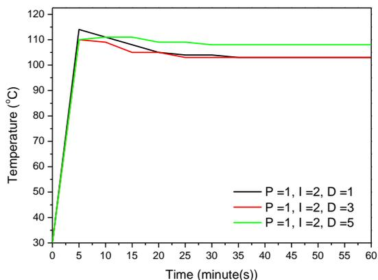
Fig. 4. Temperature responses of dehydrator while tuning PID constants
