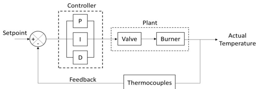
Fig. 3. Block diagram PID control of dehydrator
