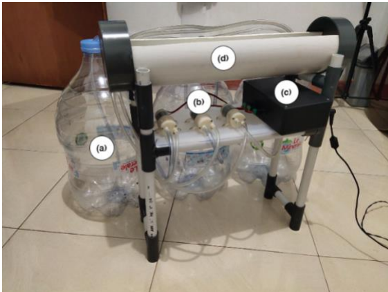
Fig. 9. The proposed system implementation: (a) the container of neutral water, pH-lowering water, and pH-increasing water, (b) water pump, (c) controller, and (d) shallot planted medium
