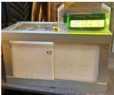
Gambar 9. Housing Baterai dan Sistem Monitoring
