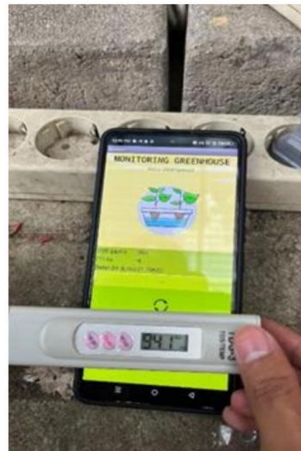
Gambar 12. Pengujian Sensor TDS
