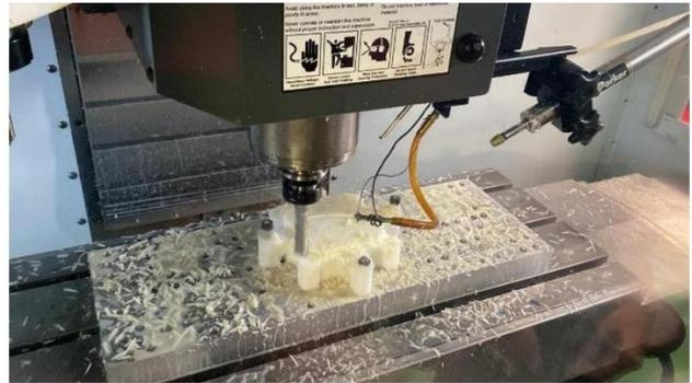
Gambar 23. Proses Permesinan Cnc Protective Upper Base
