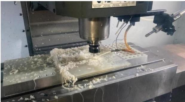
Gambar 22. Proses Permesinan Cnc Protective Upper Base
