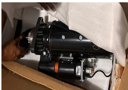
Figure 9 The process of installing a new starter dynamo on a generator engine
