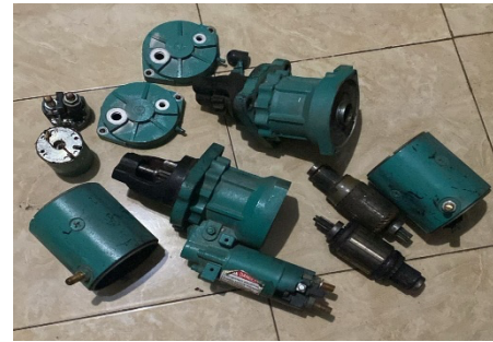
Figure 10 The old starter dynamo after being dismantled into several components
