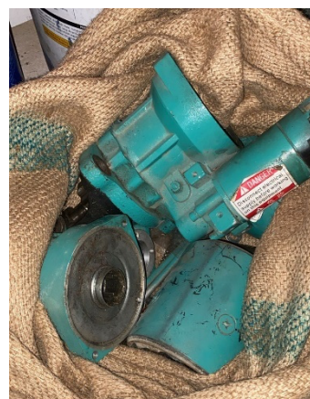
Figure 6 The old starter dynamo of the 1,000 kVA Cummins generator is damaged
