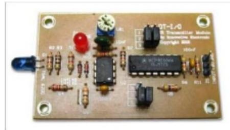
Gambar 6. Modul Infrared Transmitter
